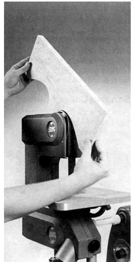
Figure 20-7. Sand odd-shaped or concave workpieces on the tracking wheel. Work in the center of the wheel.
